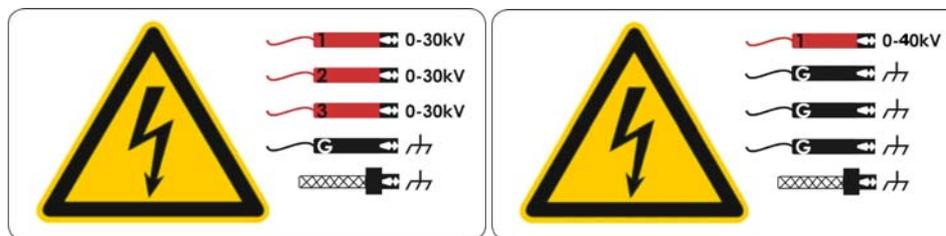
Figure 67. Lead Safety Labels – PP30 and PP85 (left) and PP40 (right).
