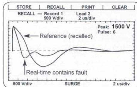
**Figure 65.** Motor with Rotor in Place and Fault Windings, Showing One Trace Shift Significantly to the Left.
