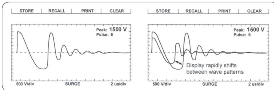
**Figure 58.** Good Wave Pattern (left) and a Representation of how a Live Wave Pattern May Appear to Move on the Display for a Winding or Coil That Contains an Intermittent Short or is Arcing (right).
