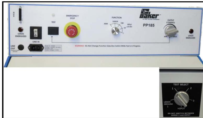
Figure 72. PP85 – 30 kV Power Pack with Three-Phase Selector Switch (Lower Right Front Panel).
