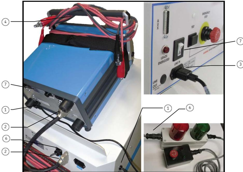
Figure 87. Power Pack Setup for Armature Tests.
