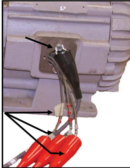
Figure 26. Attach Motor Leads to Test Leads.
