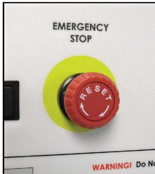
Figure 84. Emergency Stop (E-Stop) Button.
