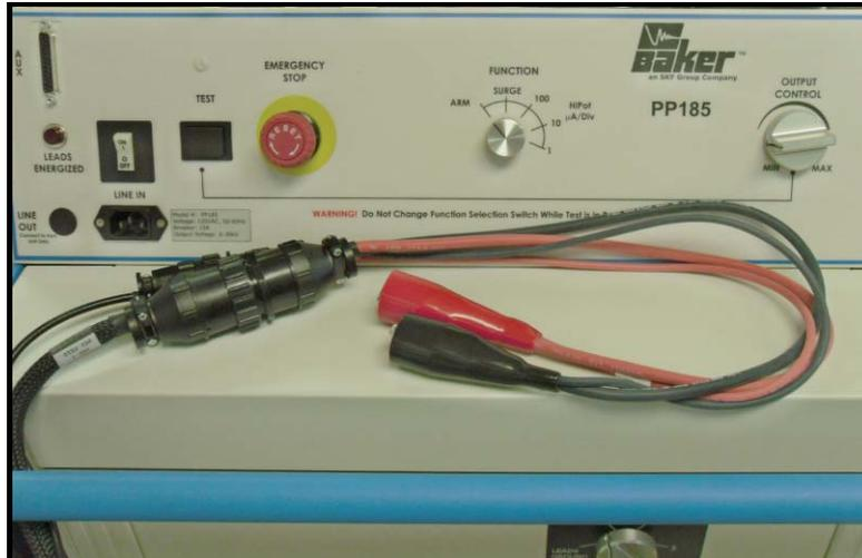
Figure 89. Accessory Clips – Inter-Pole Testing.
