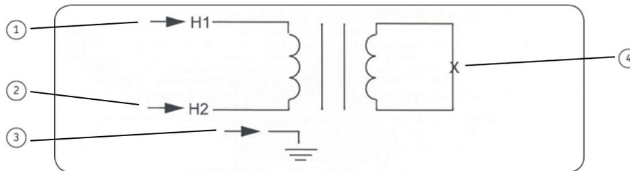
**Figure 66.** Single-Phase Transformer Connections.
