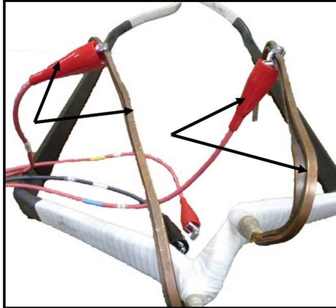
**Figure 41.** Connect Test Leads to Coil Leads.
