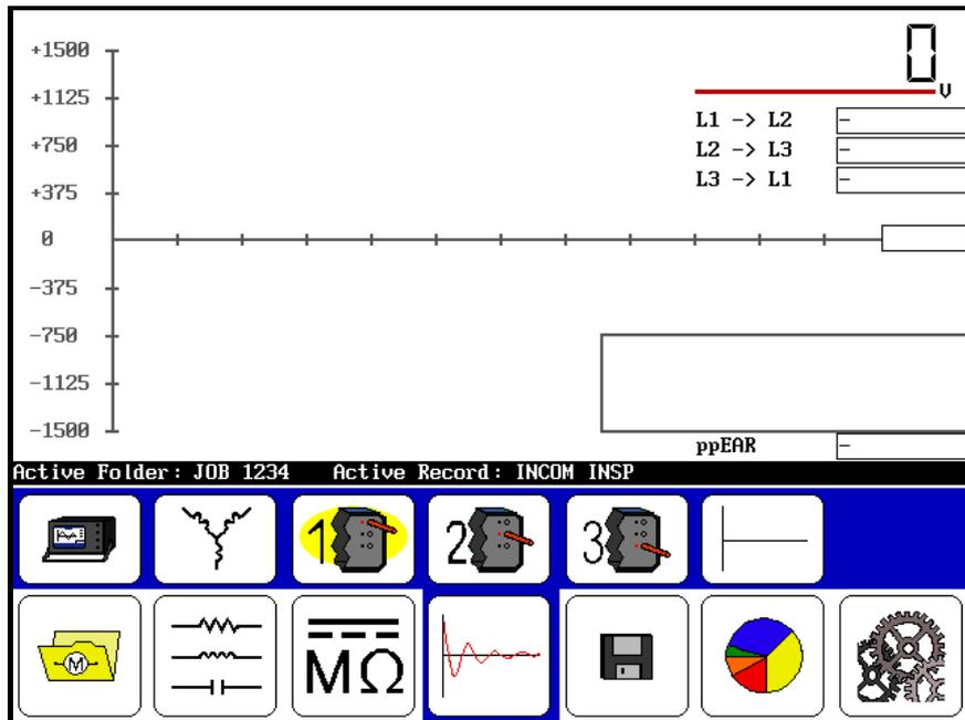
Figure 56. Surge Test Display Main Screen.
