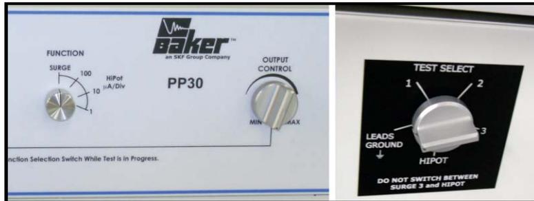
**Figure 74.** Power Pack DC-HiPot Testing Settings.
