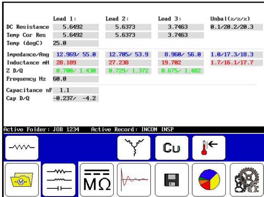
Figure 50. Completed RLC Test Screen.
