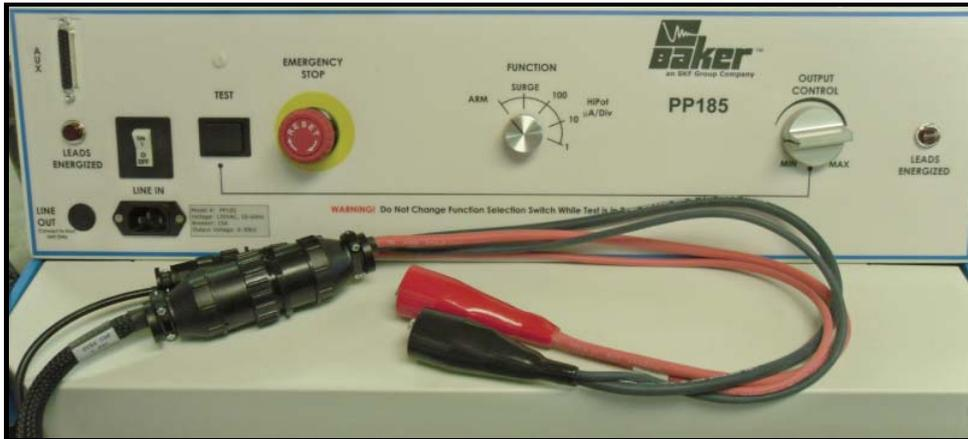
Figure 104. Connect the Clip Accessory to the Test Lead Cable .
