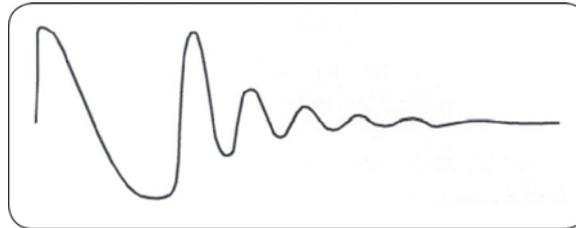
**Figure 53.** Example of a Ringing Wave Pattern Resulting from Surge Testing.
