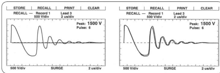
**Figure 131.** Solid Ground Coil (left) and Solid Turn-to-Turn Short (right).
