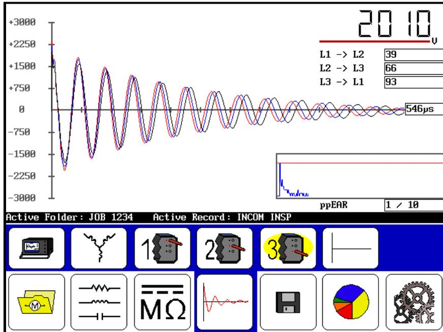
Figure 40. Completion of Winding Test.
