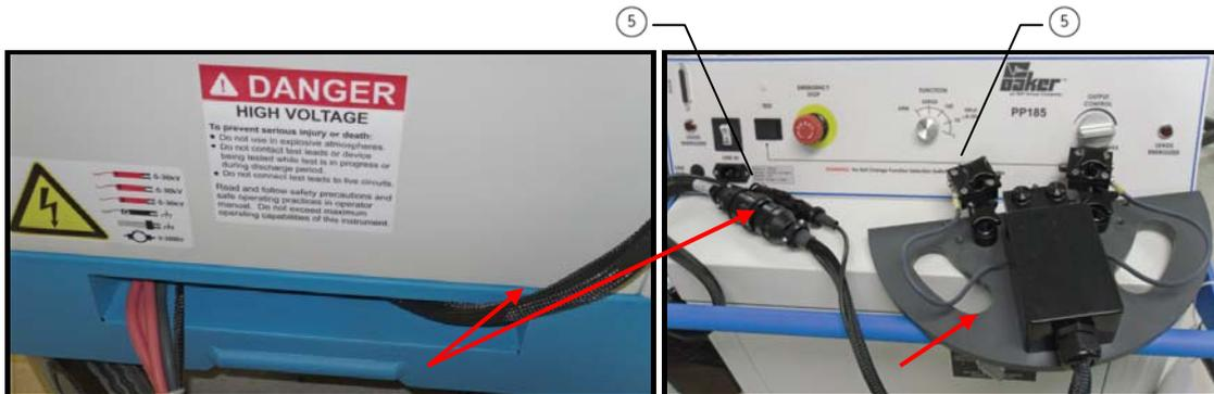
Figure 88. Test Head Cable and Connectors and Armature Fixture.
