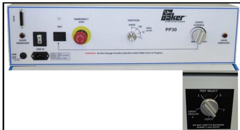
**Figure 71.** PP30 – 30 kV Power Pack with Three-Phase Selector Switch (Lower Right Front Panel).
