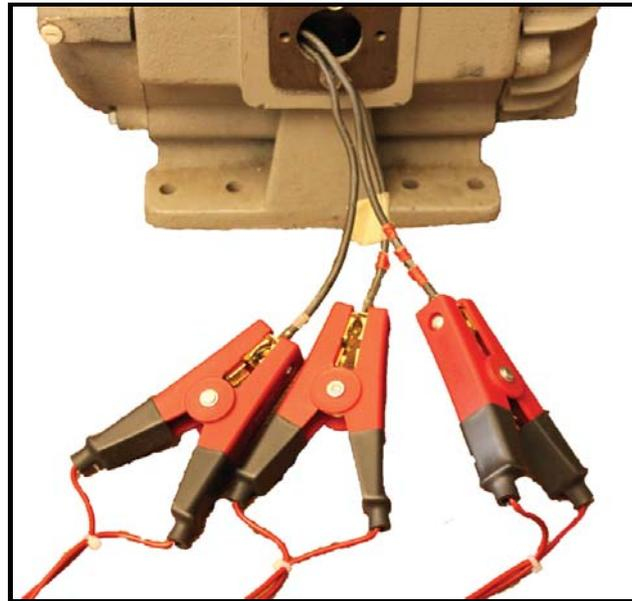
**Figure 14.** Connect RLC Test Leads to Motor Leads.
