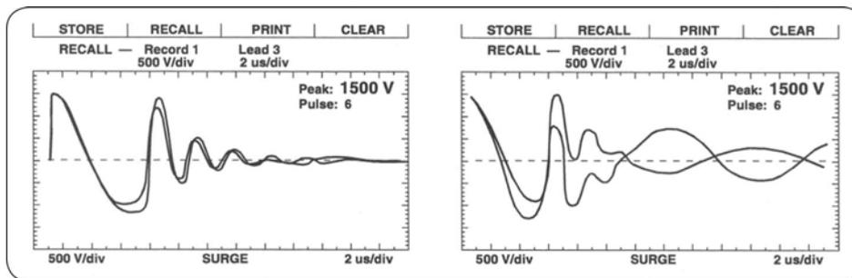
**Figure 132.** Coil-to-Coil Short (left) and Phase-to-Phase Short (right).
