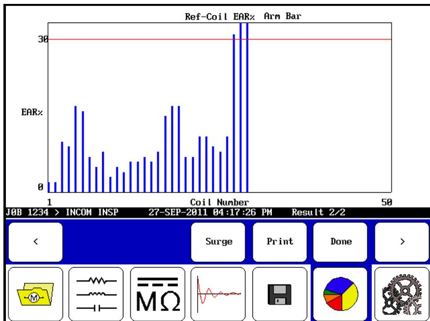
Figure 103. Commutator Coil Results Screen.
