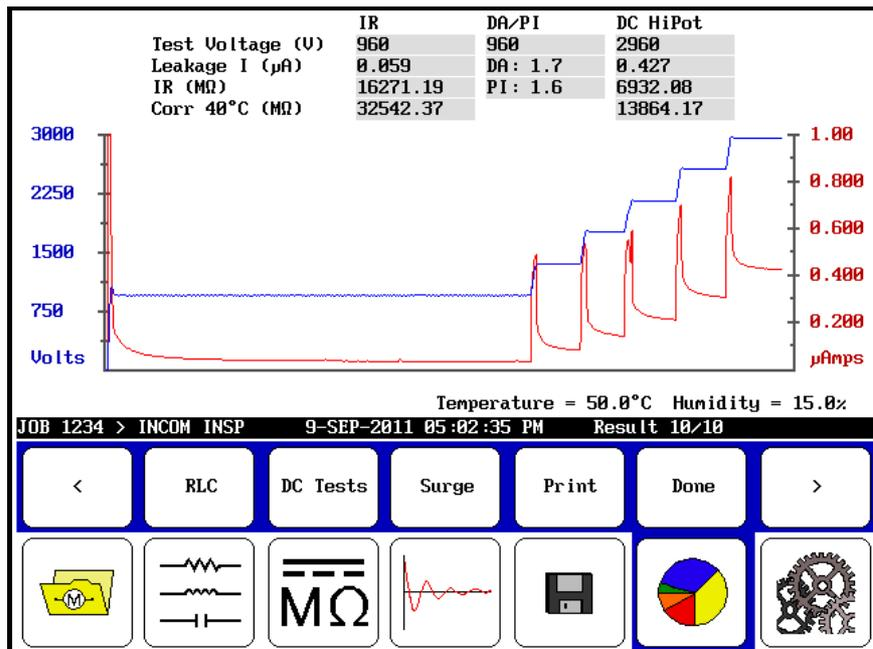
Figure 52. Completed DC Test Results Screen.
