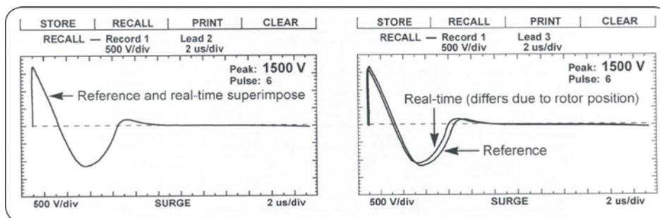
**Figure 64.** Wave Pattern Comparison for Motor with Rotor in Place.
