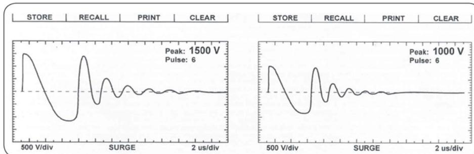
**Figure 60.** Good Coil (left) and Bad Coil (right).
