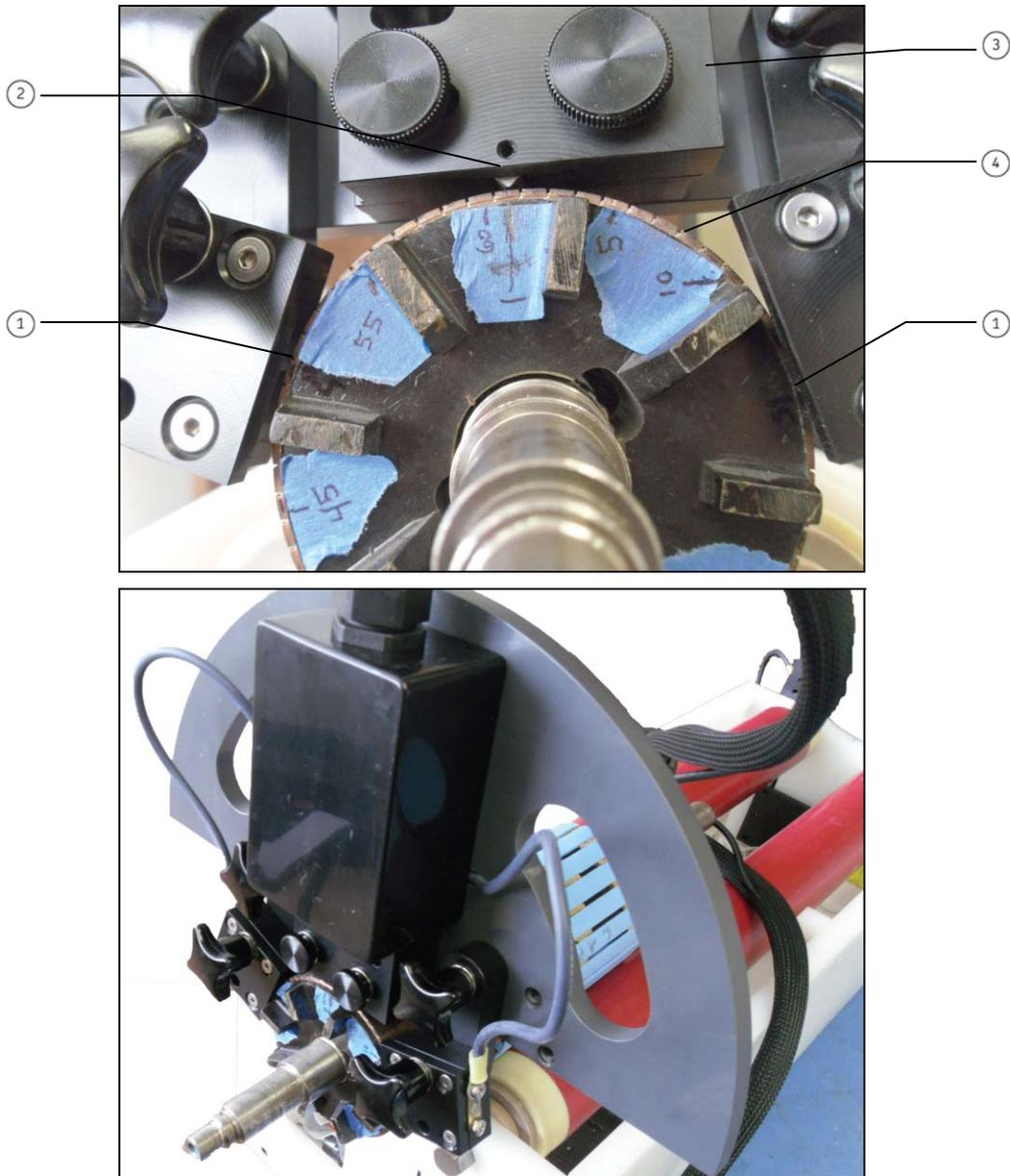
**Figure 112.** Position the Armature Fixture on the Armature.
