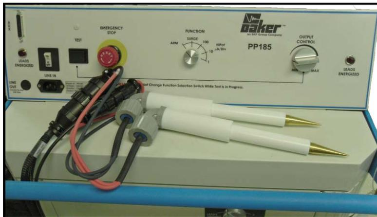
Figure 90. Accessory Probes – Armature Span Testing.
