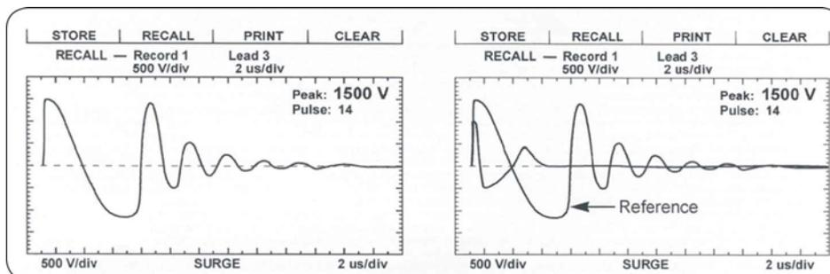
**Figure 62.** Fault Located Under the Ground Brush (left) and Fault Grounded Under the Brush or Outside of Surge Test Span (right).
