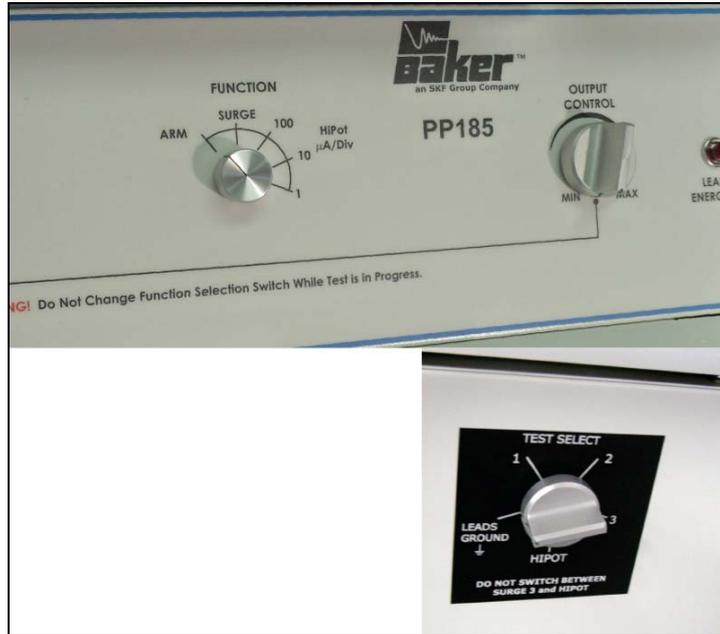
**Figure 95.** PP85 Power Pack with Three-Phase Selector Switch (Lower Right Front Panel) Set to Ground.
