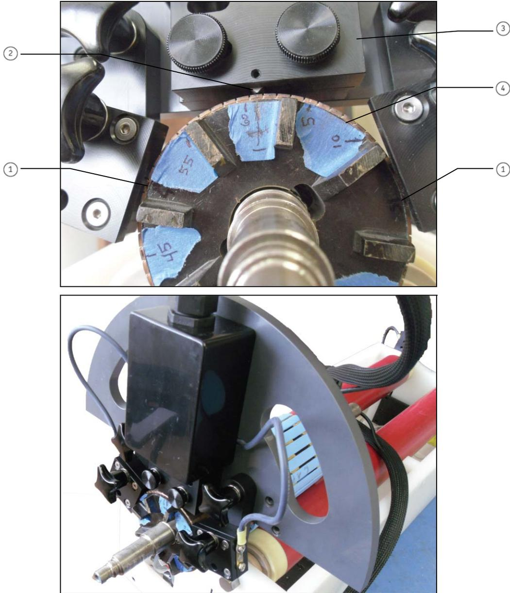
**Figure 98.** Position the Armature Fixture on the Armature.
