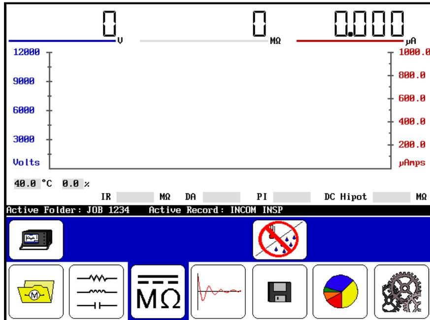
Figure 51. DC IR, DA, PI Step Voltage and DC-HiPot Tests Main Screen.
