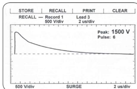
**Figure 59.** Open Phase in Lead in a Wye-Connected Motor.
