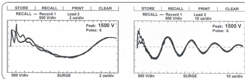
**Figure 63.** Seconds/Div Set Too Far Clockwise (left) and Adjusted Counterclockwise (right).
