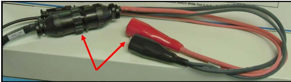
**Figure 119.** Connect Test Lead Cable to Clip Accessory.
