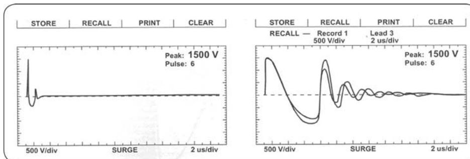
**Figure 130.** Shorted Single Winding (left) and Short Partial Ground (right).
