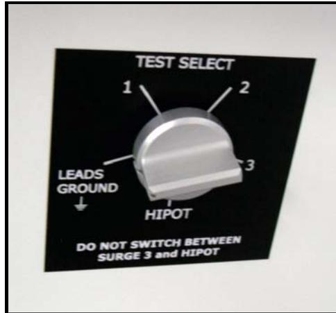
**Figure 70.** Three-Phase Lead Selector Switch with Ground Position Only on PP30 and PP85.
