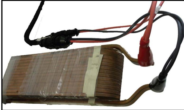
**Figure 122.** Connect Clips Accessory to DC Inter-Pole Coil.
