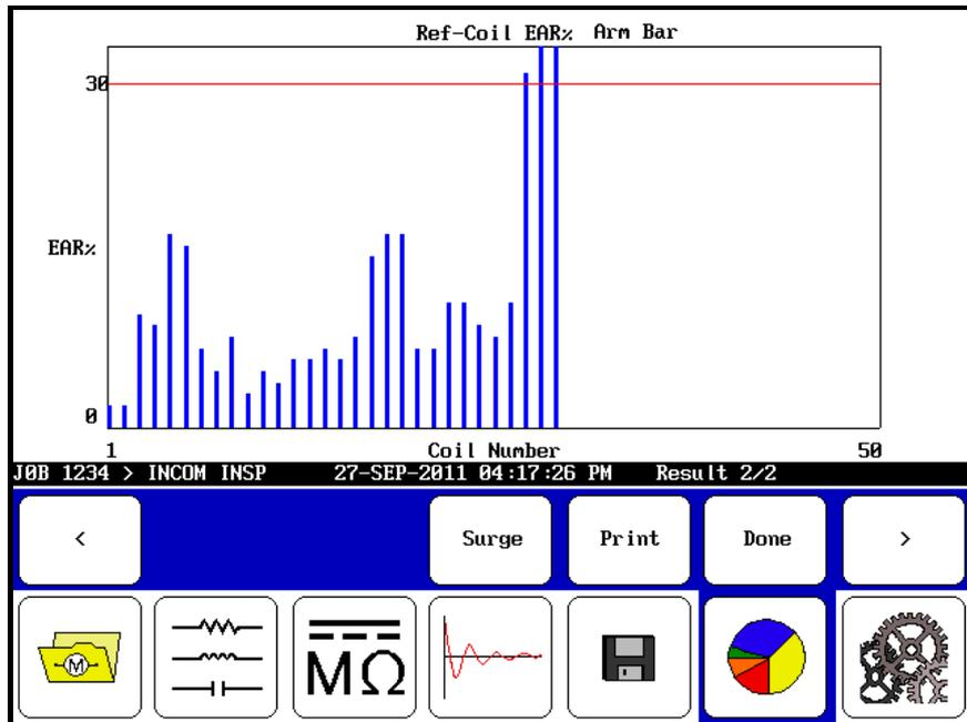
Figure 118. Commutator Coil Results Screen.
