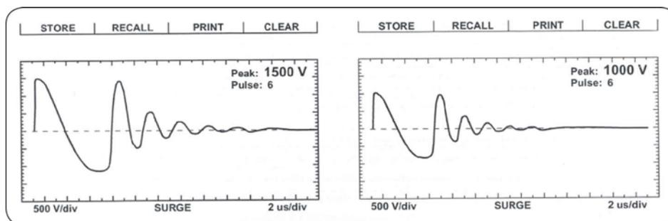
Figure 54. Good Coil (left) Versus Bad Coil (right) Waveforms.
