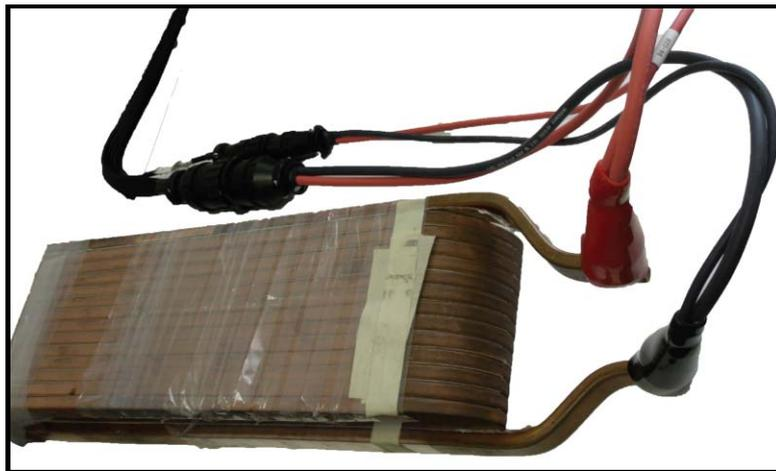
Figure 105. Connecting the Clip Accessory to a DC Inter-Pole Coil.
