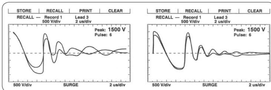
**Figure 133.** Group-to-Group Short (left) and Reversed Coil (right).
