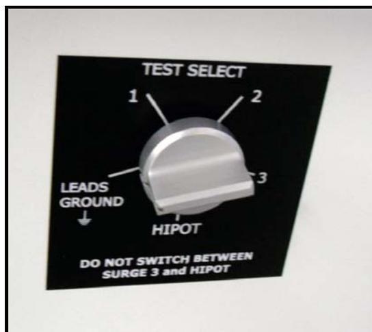
Figure 93. Three-Phase Lead Selector Switch – Ground Position.
